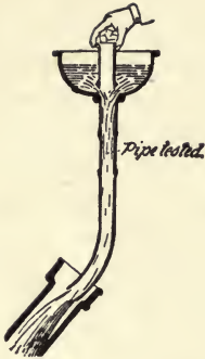
Fig. 275. Experiments on Water Flushing.
